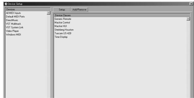
In the right side of the device setup window, select "Generic Remote" and click the "Add" button. This will add the "Generic Remote" entry to the list on the left side of the device setup window.
